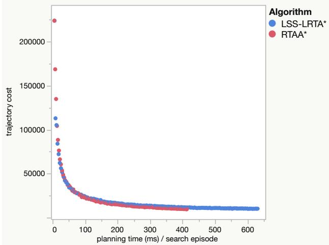
(h) mazes, unknown terrain: trajectory cost vs planning time / action execution (see Appendix A for log scale)
