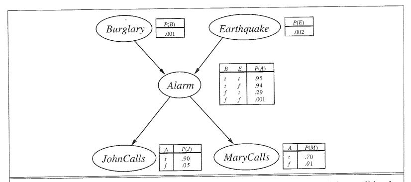
**Figure 14.2** A typical Bayesian network, showing both the topology and the conditional probability tables (CPTs). In the CPTs, the letters B, E, A, J, and M stand for Burglary, Earthquake, Alarm, JohnCalls, and MaryCalls, respectively.
