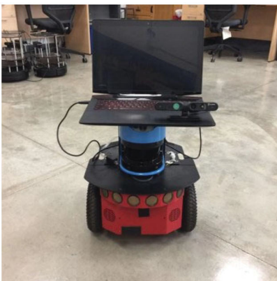
Figure 1. Pioneer 3DX platform as a SAR for dementia-care.
