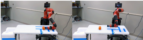
Fig. 9: Experimental setup for the cylinder rolling task. The cylinder is placed at a designated starting point and the robot attempts to roll the cylinder into the basket at the end of the table.
