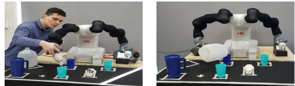
(a) Kinesthetic teaching of the (b) Yumi robot performing tea-making task to a Yumi robot. Adding Milk action.
