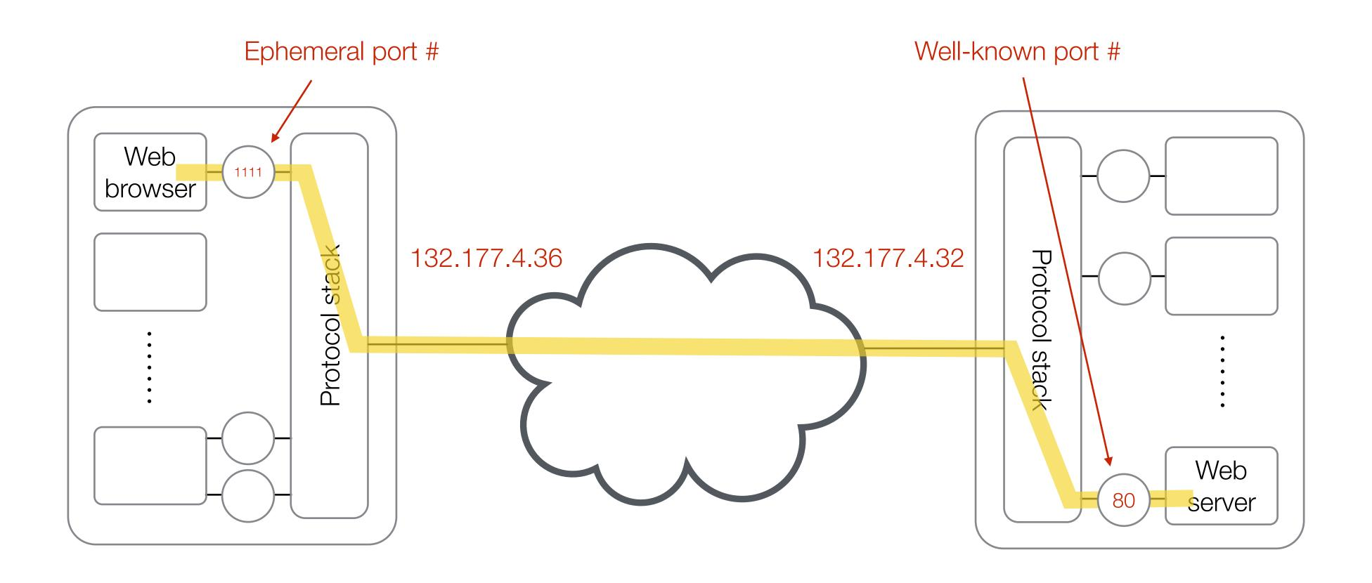
A process (web browser) connected to ephemeral port 1111 on a host with IP address 132.177.4.36 opens connection to a process that listens on well-known port 80 (web server) on a host with IP address 132.177.4.32
