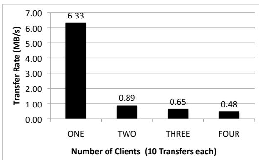
Figure 9: Normal user's transfer rate changes as the number of other clients retrieving large data files for multiple large users increases. (Limited gateway connection bandwidth)
