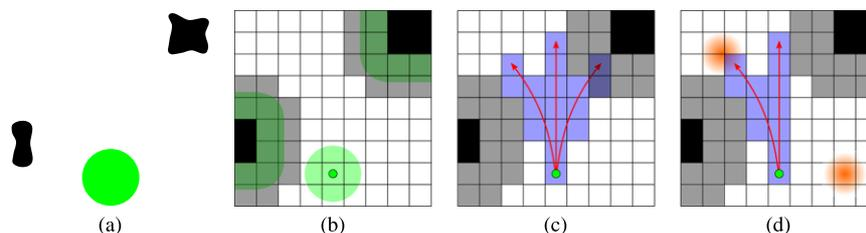
Fig. 1. Generating the search space using (b) discretization, (c) motion primitives and collision checking and (d) dynamic obstacles. (Colors are visible in the online version of the article; <http://dx.doi.org/10.3233/AIC-140604>.)
