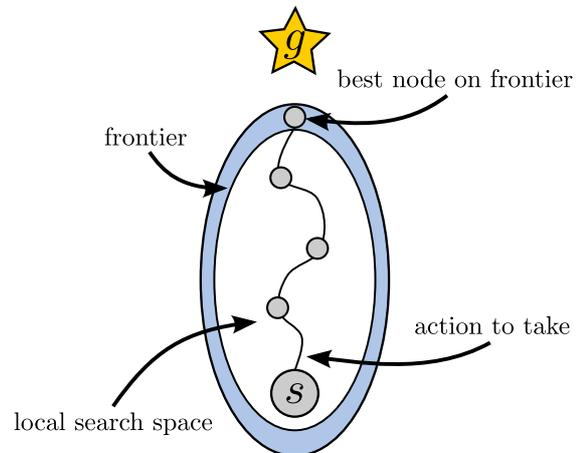
Fig. 6. The local search space and frontier of an iteration of LSS-LRTA\*. The best node on the frontier and the corresponding action to take are shown. (Colors are visible in the online version of the article; <http://dx.doi.org/10.3233/AIC-140604>.)
