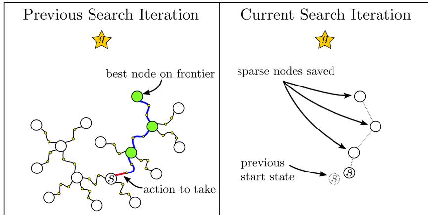
Fig. 4. Path saving across iterations of RTR\*. (Colors are visible in the online version of the article; <http://dx.doi.org/10.3233/AIC-140604>.)
