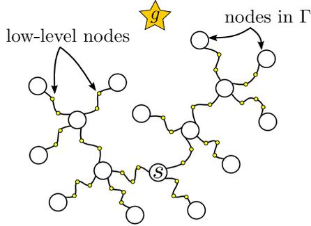
Fig. 3. The nodes in  $\Gamma$  (large, white) and the nodes in the low-level state space (small, yellow) that are explored by an  $R^*$  search with  $k = 3$ . (The colors are visible in the online version of the article; <http://dx.doi.org/10.3233/AIC-140604>.)
