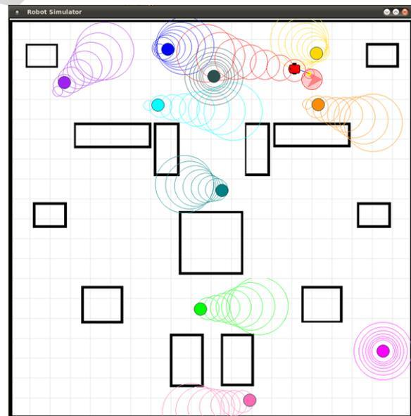
Fig. 7. The simulator used showing the dynamic obstacles (filled circles), the robot (red filled circle), and the goal (light red filled circle with arrowhead, near robot). Hollow circles indicate probability distributions over predicted future trajectories of obstacles. (The colors are visible in the online version of the article; <http://dx.doi.org/10.3233/AIC-140604>.)
