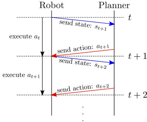
Fig. 2. The interaction between the robot simulator and each planner. (Colors are visible in the online version of the article; <http://dx.doi.org/10.3233/AIC-140604>.)
