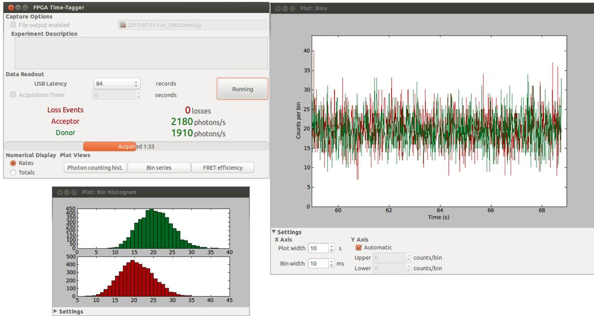
Figure 2: The `timetag_ui` interface during data acquisition
