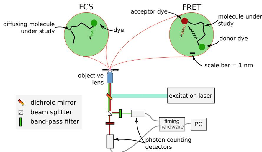
Figure 1: A schematic representation of a typical fluorescence spectroscopy experiment. The bubble on the left shows a diffusing singly-labelled molecule as might be used in an FCS experiment. The right bubble shows a pair of dyes undergoing energy transfer, as would be seen in a FRET study.
