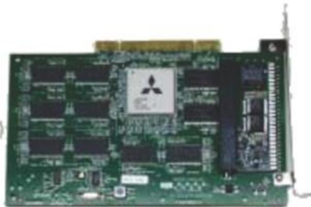
**Figure 1.21:** The VolumePro PCI card
