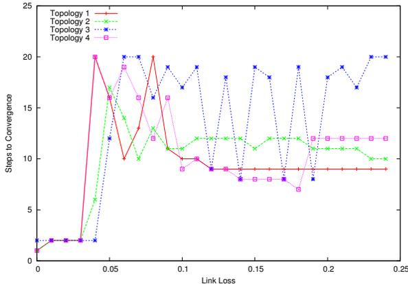
Figure 2: Cycles required to stabilize the RTL.
