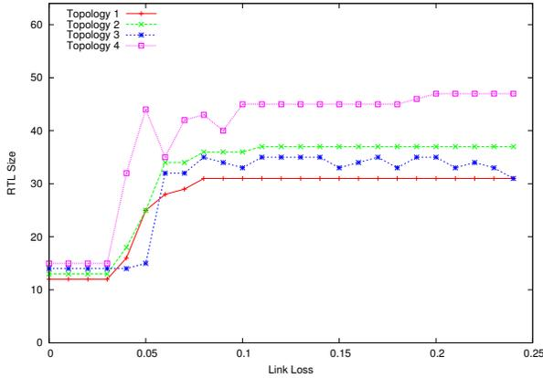
Figure 1: RTL size for varying link losses.
