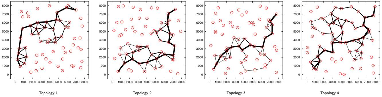
Figure 3: Connections representing the possible paths of packets for RTLs in 3 cases of link loss. The thickest lines represent the RTL under 0% link loss, (shortest path), while the thinnest represent the RTL under 24% link loss.
